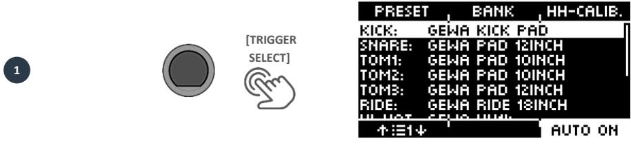
Start the calibration and press the button [F3] "HH-CALIB."
