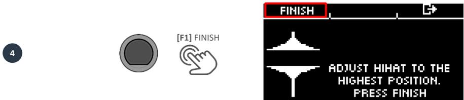
Now the hi hat is fully calibrated and playable. With the hi hat symbol you can directly test whether the mechanism works. Then confirm the setting by pressing the button [F1] "DONE"
