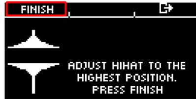
Now the hi hat is fully calibrated and playable. With the hi hat symbol you can directly test whether the mechanism works. Then confirm the setting by pressing the button [F1] "DONE"
