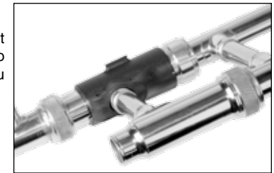
Shown: Bushing with both shims in place. It's now ready to be applied to the instrument.
