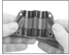
Shown: Bushing with both shims in place. It's now ready to be applied to the instrument.
